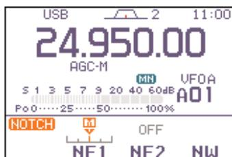
⚡ While adjusting the manual notch filter, noise may be heard. This comes from the DSP unit and does not indicate an equipment malfunction.
