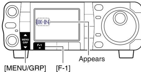
When using a paddle, set “**Key Speed**” in the quick set mode to adjust the keying speed. (p. 124)
