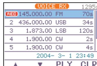
The voice recorder stores the received audio in 15 sec. blocks. Thus the total recording time is reduced by 15 sec. each time recording is stopped.
