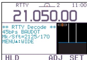
The transceiver has an RTTY decoder for Baudot (mark freq.: 2125 Hz, shift freq.: 170 Hz, 45 bps).
