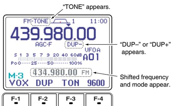
To set the transceiver for repeater operation, follow the steps ① to ③ to select VFO mode, desired band, FM mode.
