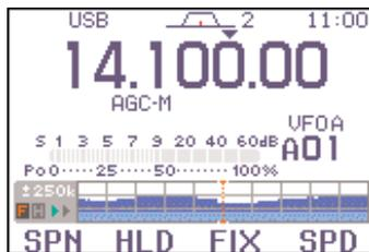
**NOTE:** If there is a lot of signal noise, turn the pre-amp OFF and the attenuator ON (p. 74) to reduce the input level and improve the readability of the scope.
