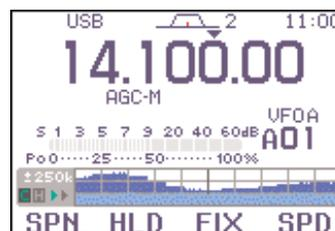
NOTE: If there is a lot of signal noise, turn the pre-amp OFF and the attenuator ON (p. 74) to reduce the input level and improve the readability of the scope.
