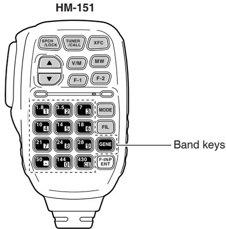
The triple band stacking register provides 3 memories in one band. 3 sets of frequency and operating mode on each band are automatically stored when used.
