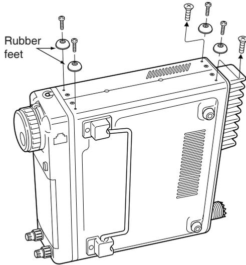
② Attach the MB-106 to the left side of the transceiver as shown below.
