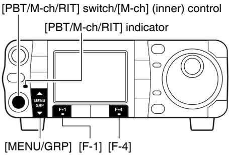
[PBT/M-ch/RIT] switch/[M-ch] (inner) control
