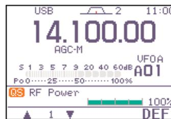
If a linear amplifier is connected such as the IC-PW1/EURO, set the output power using the ALC meter (see below) to the ALC zone (ALC meter reading should be within this zone), otherwise the linear amplifier will not work properly.
