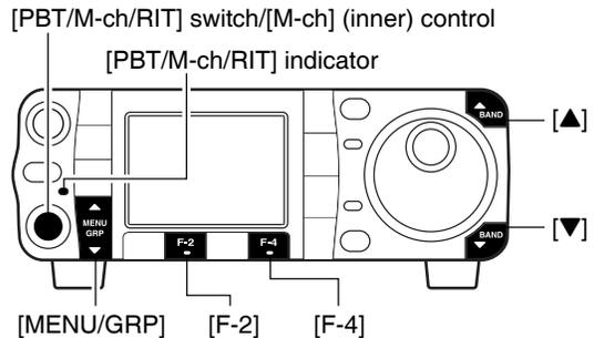
[PBT/M-ch/RIT] switch/[M-ch] (inner) control
