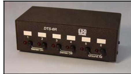
The DTS-6 handles up to 1500 watts PEP (250 watts on 6 meters) of RF power, and can be used with any coax-fed antenna. The Radio Sense feature needs at least 2 volts from your rig, at negligible current. The DTS-6 features standard SO-239 connectors, and requires an external 12 vdc power supply at 500 ma. If the external power supply fails, all inputs are automatically grounded, so it's fail-safe. Switching is done by rugged, sealed industrial relays.
