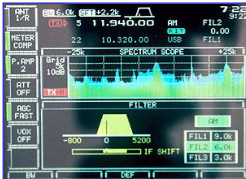
With Mini-Scope ON, a menu (or the bar-graph meter) displays in the lower field. The scope "shrinks" and displays in the centre field. With Mini-Scope OFF, display is identical to IC-756Pro II (right).
