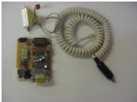
Programming board for the micro Display to 817 cable DB25 is a programming lead for the EEPROM
