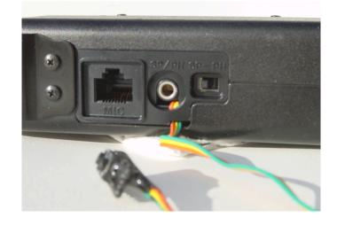
□ Solder the switch assembly to the ADSP2 board
