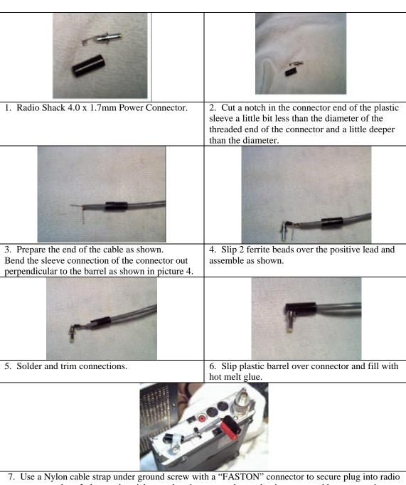
power socket. I also used a stick on nylon tie wrap anchor and a tie wrap to add more security.
