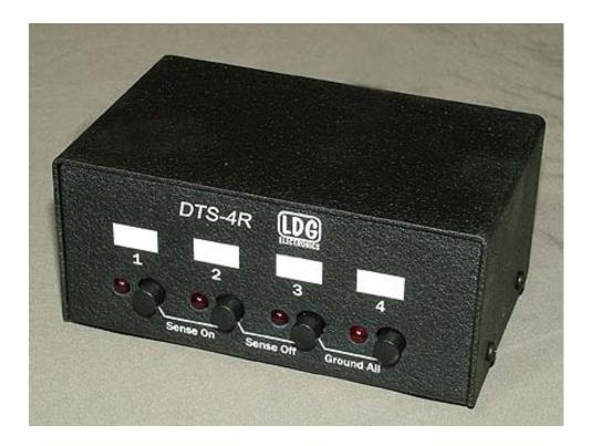
The DTS-4R remote is smaller than the DTS-4, but has the same four switches and four LED lights on the front. On the back, it has the same power, radio sense and control jacks, but no coax connectors.
