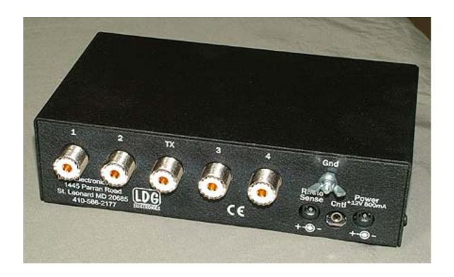
The 2.5 x 5.5 mm jack coaxial DC power connector is on the right. The ground connection is via the wingnut. The radio sense input is a second  $2.5 \times 5.5 \text{ mm}$  coaxial jack, and the control cable is a 1/8" stereo jack; the control cable is included with the DTS-4R remote.
