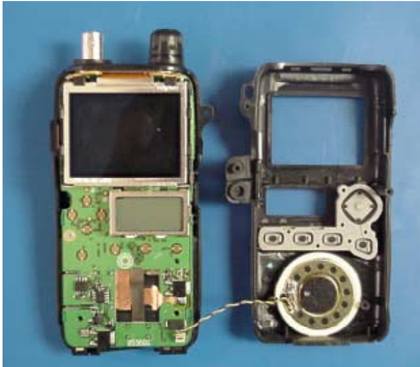
FRONT VIEW OF PCB SHOWING SPEAKER CONNECTION TO TOP COVER
