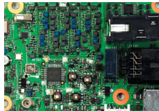
Icom original DDS circuit
